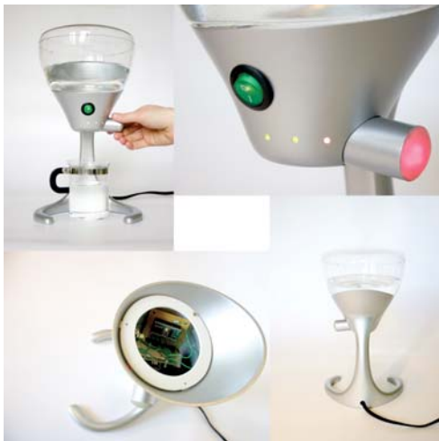
Figure 4. Prototype of the on-demand kettle with BS2 microcontroller hidden into it.
